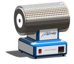
Tubular furnace with temperature controller for laboratory
